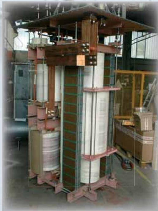
Voltage shield regulator - active part
